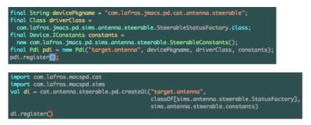
Fig. 3: Deployment code - JMaCS (top) vs MaCS
